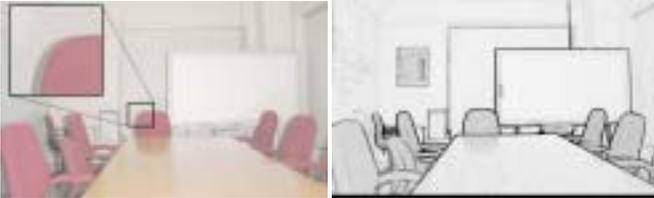
Figure 15: Room sized scene: Right flash image and depth edge map.
