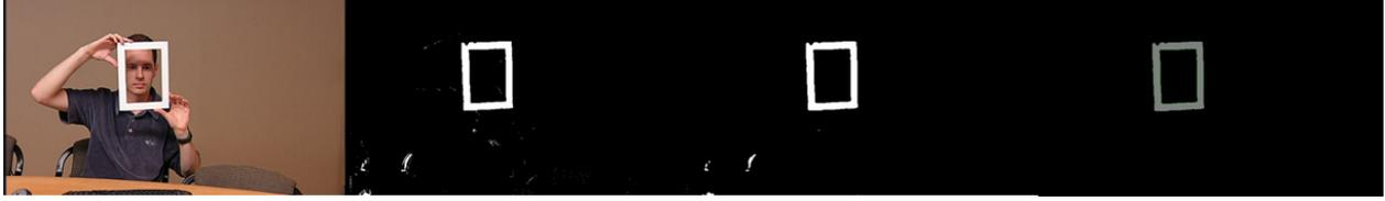
Figure 2: Target finding stages: Source, Color Match, Threshold/Filter, Region growing
