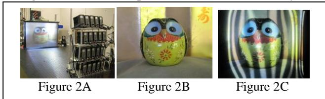
Figure 2A depicts a 20-projector system. Figure 2B shows a test image that we use to evaluate the characteristics of our C3D system. Figure 2C shows the banding artifact that we observed
