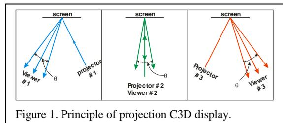
Figure 1. Principle of projection C3D display.
